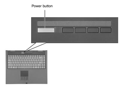
The power button is preset to On/Off mode. However, you can also set it to function in Standby/Resume mode. For instructions on changing the power button mode, see "Changing power settings" on page 131.
