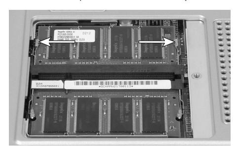
**7** Pull the memory module out of the slot.
